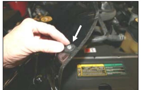
**12.** Install the tall grommet (#12) with the groove at the top, into the hole in the Cool Air Dam (#3). Next push the supplied aluminum sleeve (#10) into the hole in the grommet as shown.
