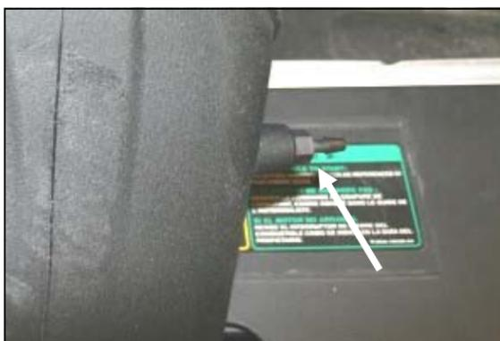
8. Install the 1/8"NPT x 3/16" barbed fitting (#13) into the small threaded hole in the side of the Airaid Intake Tube.
