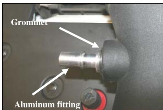
7. Install the provided grommet (#11) into the large hole in the side of the Airaid Intake Tube (#2). Next, carefully install the supplied aluminum fitting (#14) into the grommet as shown.
