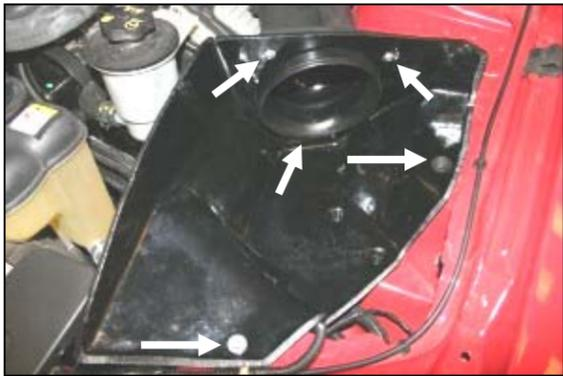
**13.** Install the Cool Air Dam into the vehicle aligning the grommet posts on the bottom of the CAD into the factory grommets in the fender well. Now install three 1/4" button head bolts (#6) and flat washers (#7) thru the CAD and into the Airaid Intake Tube. Next reinstall the factory bolts from step #1, and step #6 into their respective holes.
