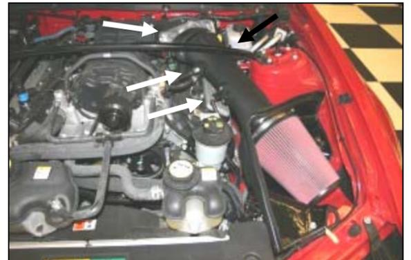
**15.** Adjust the Airaid Intake Tube for fit and then tighten the hose clamps on the throttlebody and the tube. Now reconnect the wiring harness to the MAF, the breather to the aluminum fitting, and the vacuum hose to the barbed fitting on the Airaid Intake Tube.
