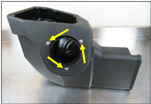
12. Install the Filter Adapter onto the Cold Air Box as shown using the three 1/4-20 Button Head Screws and 1/4" Flat Washers.
