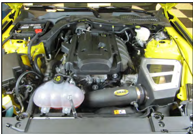
21. Double check your work. Make sure all clamps, hoses, bolts, and screws are tight. Double check the hood clearance. Reconnect the negative battery cable and reinstall the cover.
