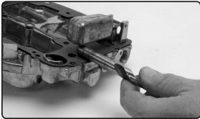
Checking float level with a 7/16" drill bit
