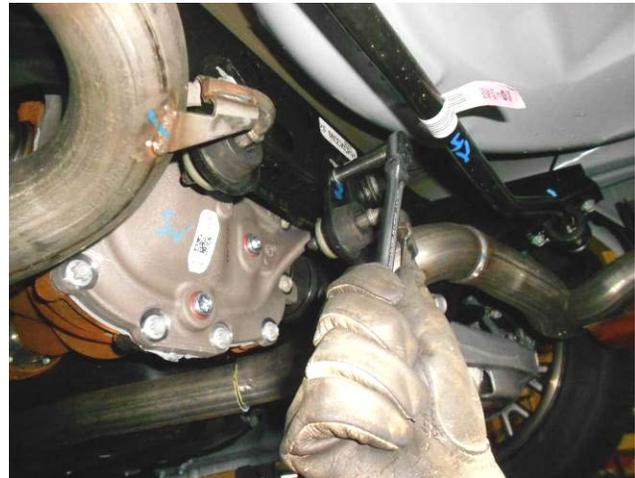
2) Support both of the mufflers at the rear of the system with a stand. Then using a 13mm wrench, unbolt the two hangers located just behind the rear differential from the cross member, leave them attached to the factory exhaust system. Again using a 13mm wrench, unbolt the hangers at the rear of the vehicle from the frame and leave attached to the system.
