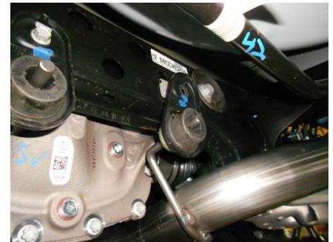
3) Place the right muffler assembly **#815430-403** up into position and slide the inlet onto the Y-pipe approx. 2.00". Support the assembly with a stand and remount the rear hanger mount to the frame, tighten securely. Remount the front hanger to the cross member and tighten securely. Leave the clamp on the inlet loose for now. Repeat this step with muffler assembly **#815430-402** on the left side of the vehicle.
