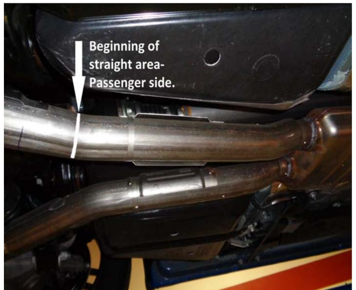
4) Behind the factory center resonator, follow the pipes back just past the second bend of each pipe, make a mark on each pipe where the bend ends and the straight area begins. See above photos.
