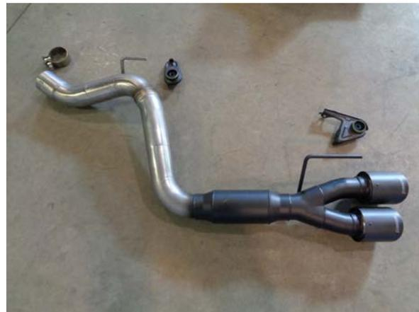
1) Place the new Flowmaster muffler units next to the factory units and swap the front and rear hanger mounts from the stock mufflers to the Flowmaster assemblies. Also, place a provided 2.50" clamp onto the inlet of each assembly. Tighten the clamp just enough to hold in place.
