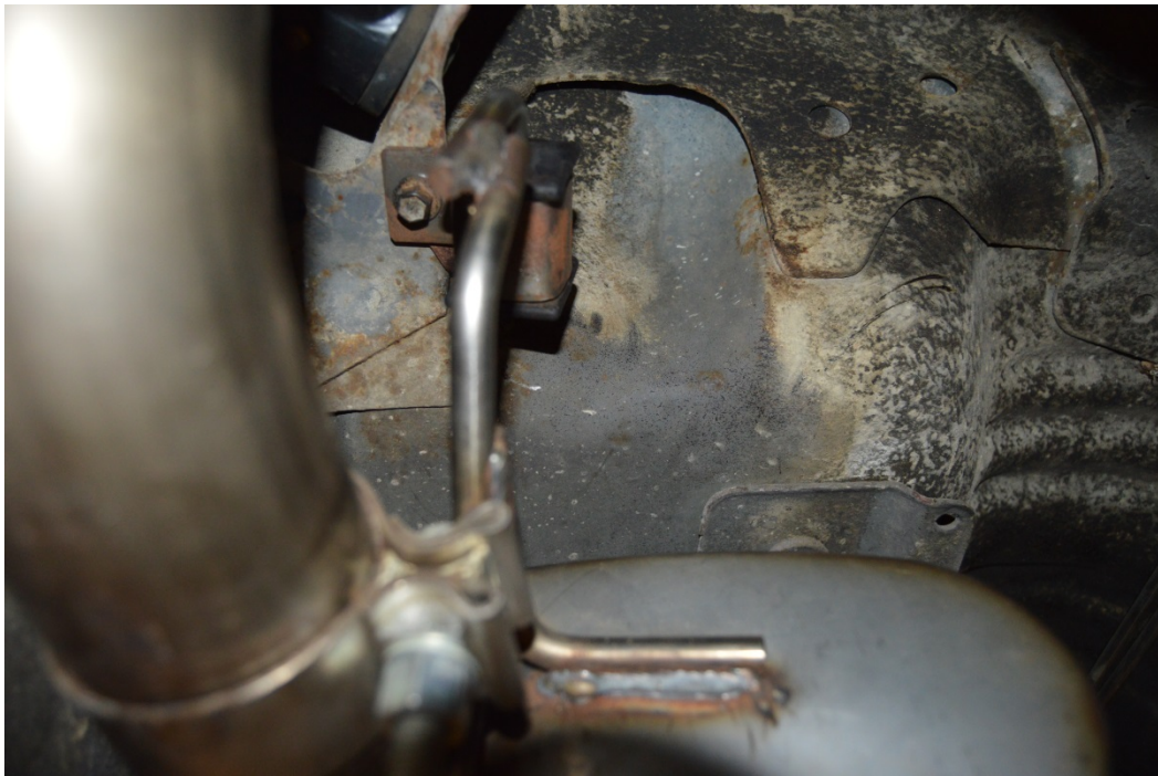
Drivers side hanger location above over axle tube on upper control arm structure.
