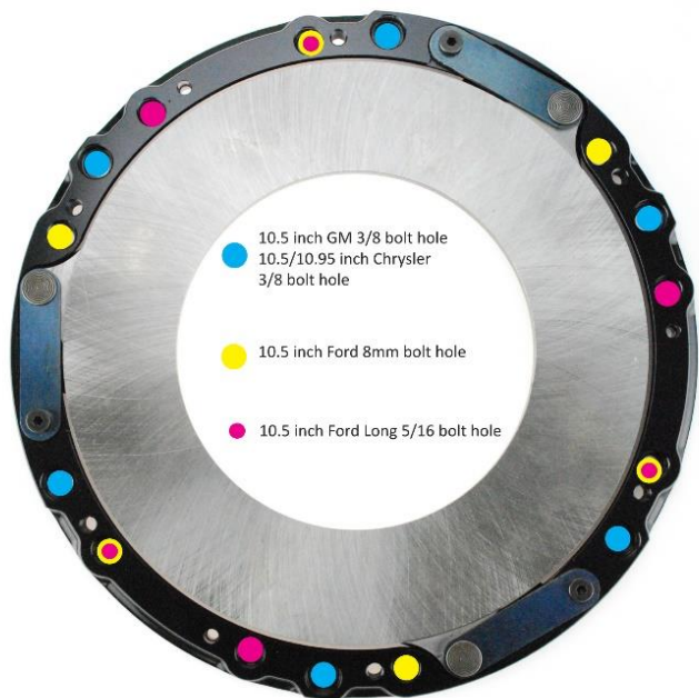
10.5 inch ring mounting configurations
