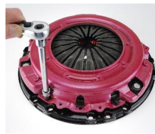
Removing 6 – cover bolts
