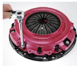
Removing 6 – cover bolts
