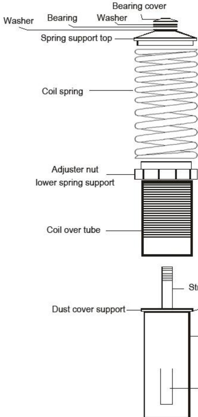
**Complete coil over assembly mounts under strut tower in wheel well!**
