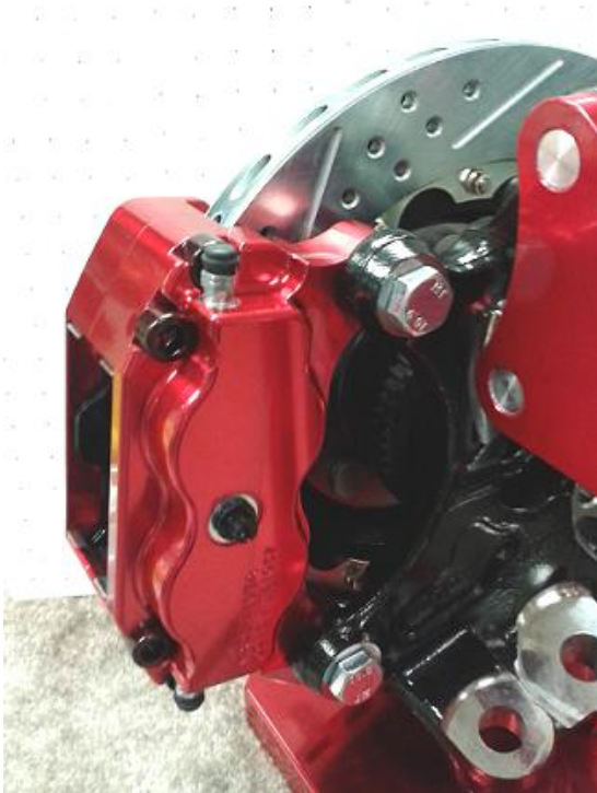
Figure 1: Caliper installed (inboard view)
