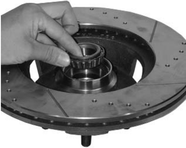
Figure 1 – Inner Wheel Bearing Installation
