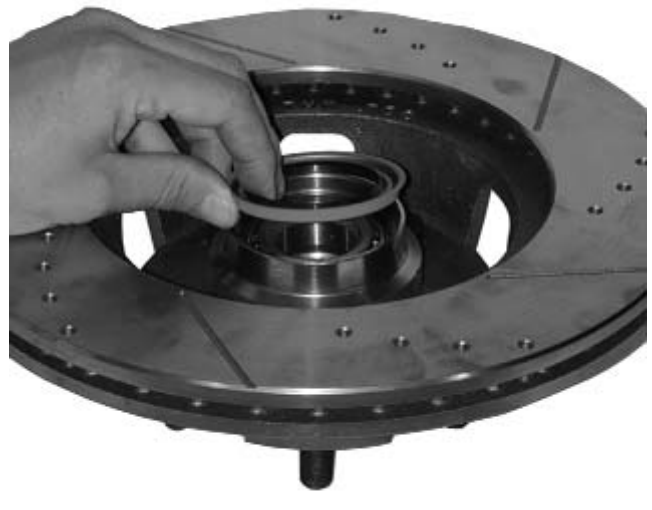
Figure 2 – Inner Wheel Seal Installation
