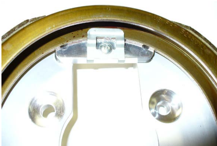
Figure 4 – Installed Park Brake Shoe Upper Retainer
