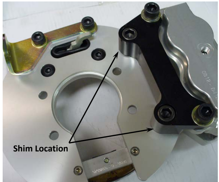
Figure 6b - Shim Location
