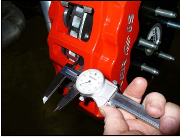
Figure 6: Measurements taken in order to shim
