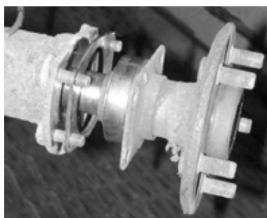
Installation of Spacer Plate.
