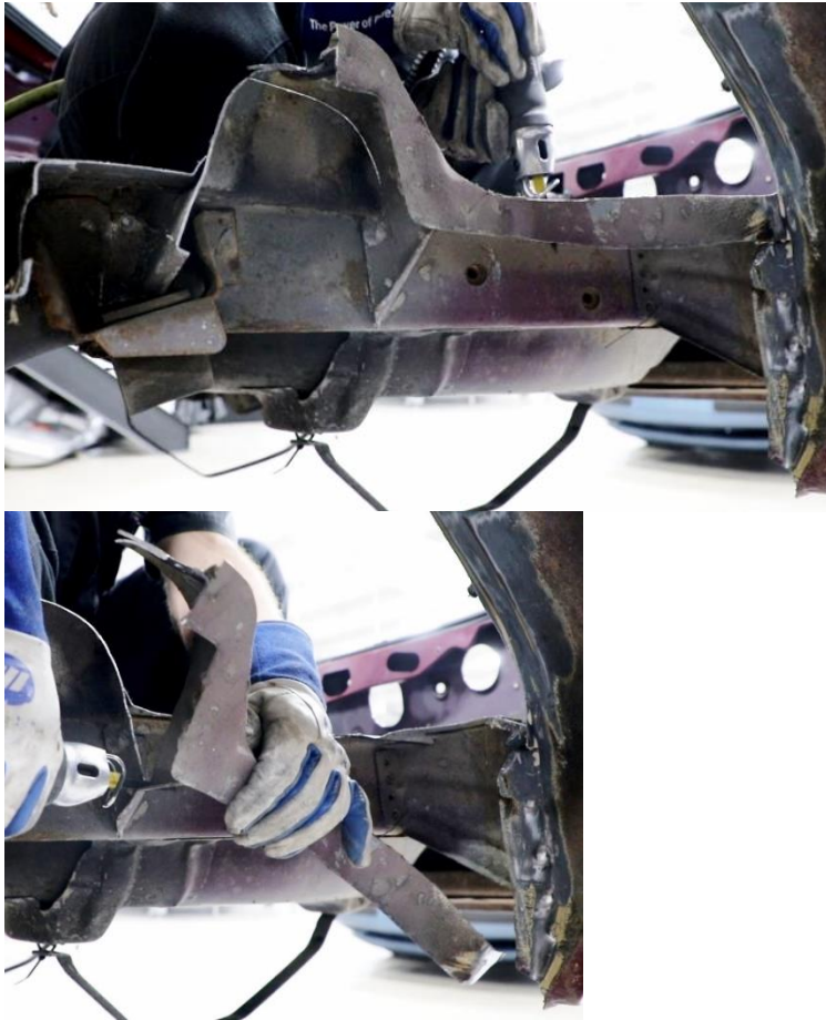
Figure 20 – Remove Rear Factory Structure
