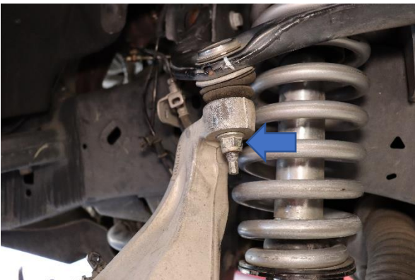
Step 4. Loosen the upper ball joint nut.
