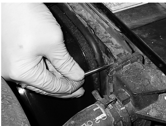
Install temp. probe near inlet hose...
