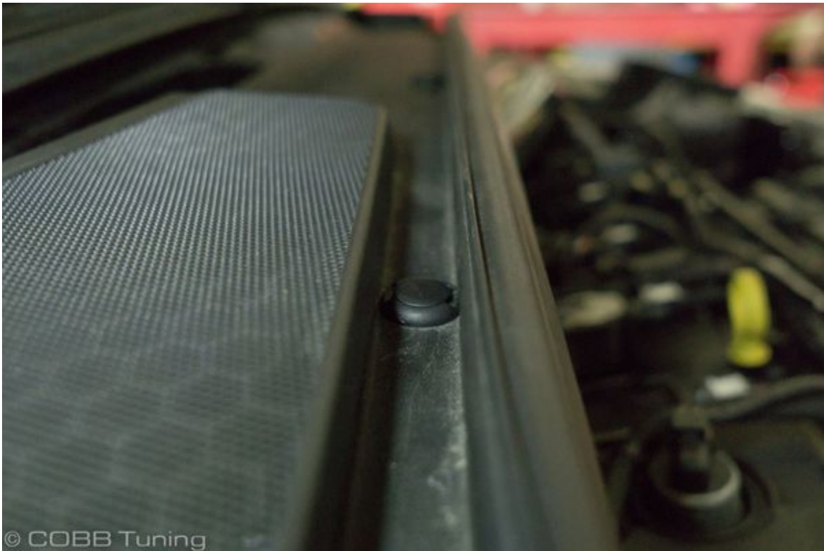
20. Reinstall the engine cover by merely applying downward pressure from the top.
