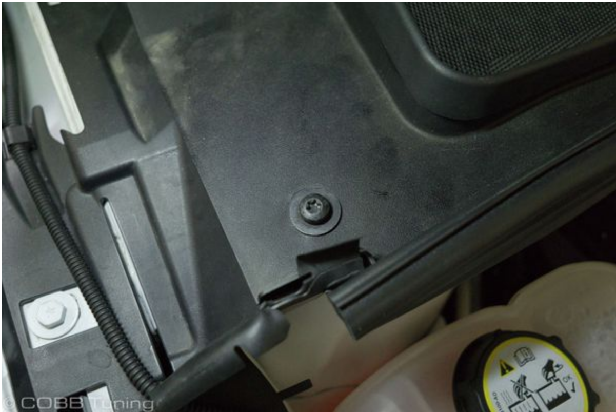
18. Secure the upper and lower cowl portions on the driver's side with the OEM bolt.
