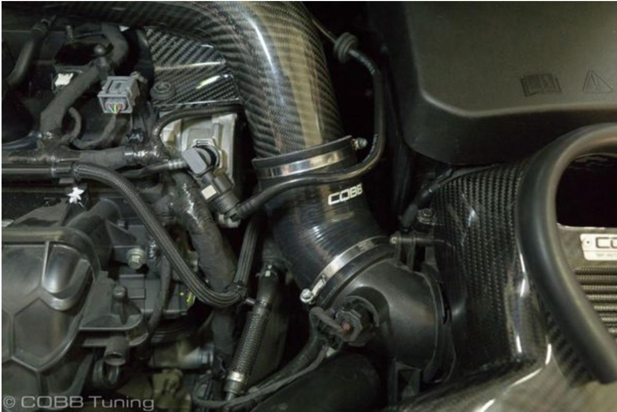
8. Attach the intake tube bracket to the engine using the supplied 6mm x 25mm flanged hex bolt.
