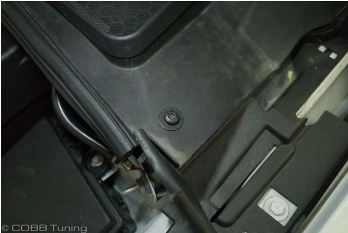
19. Finish securing the upper cowl by reinstalling the (4) OEM push pins along the forward edge.
