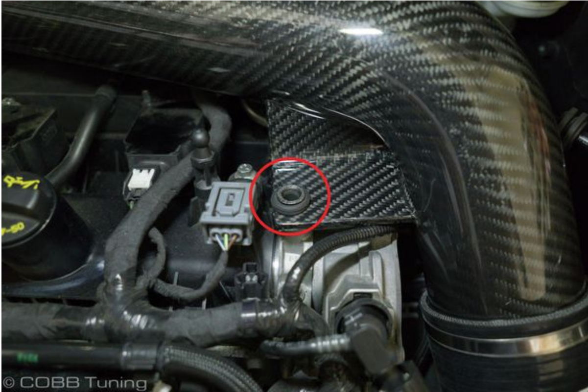
8. Attach the intake tube bracket to the engine using the supplied 6mm x 25mm flanged hex bolt.
