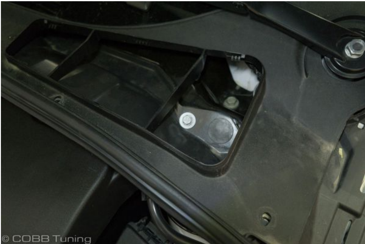
14. Secure the lower cowl debris guard on the passenger's side with the OEM bolt.
