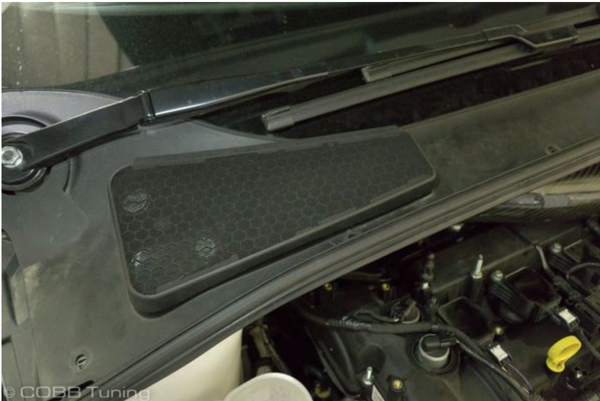
16. Reinstall the driver's side upper cowl debris guard by pressing it on until you hear it click.
