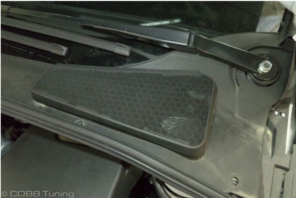
17. Secure the upper and lower cowl portions on the passenger's side with the OEM bolt.
