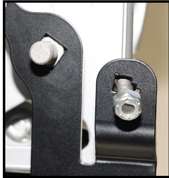
Pedal with carriage bolt and nut.
