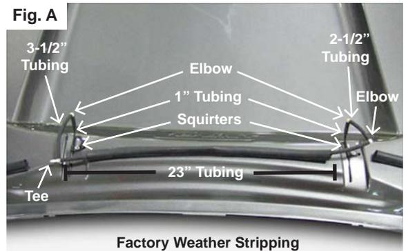
STEP 7: After all adjustments have been made, reinstall the weather stripping on the rear of the hood. You will need to cut it so that it does not cross over top of the squirter. Cut the factory squirter hose before the first squirter connection **as shown in fig.B.** Then, run the squirter hose through the weather stripping and connect it to the squirter **as shown in fig.C.** (You may need to bend the squirter into position.)
