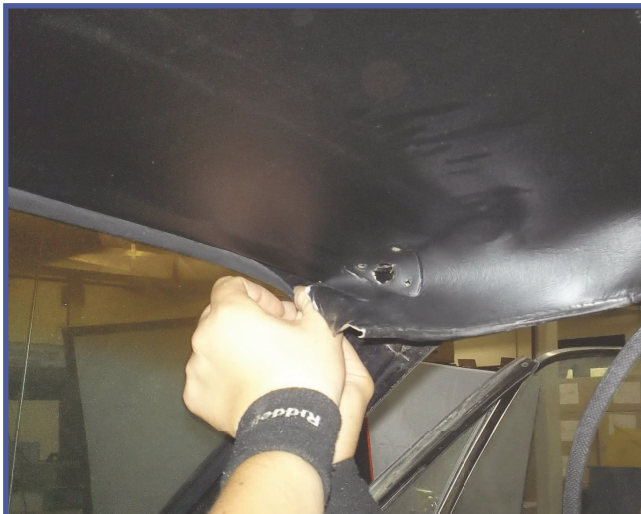
1. Pull material away from window rubber seal
