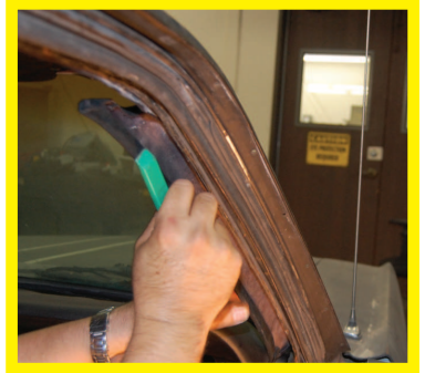
Using the Plastic Trim Tool, tuck the A-Pillar cover into the windshield window seal.
