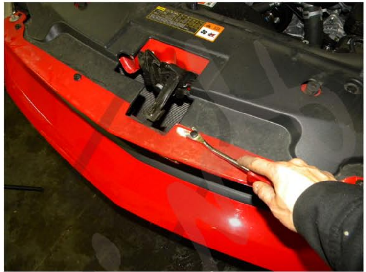
6. Remove the (4) plastic clips
