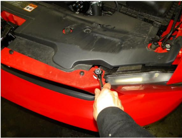
5. Remove the (2) 8mm screws
