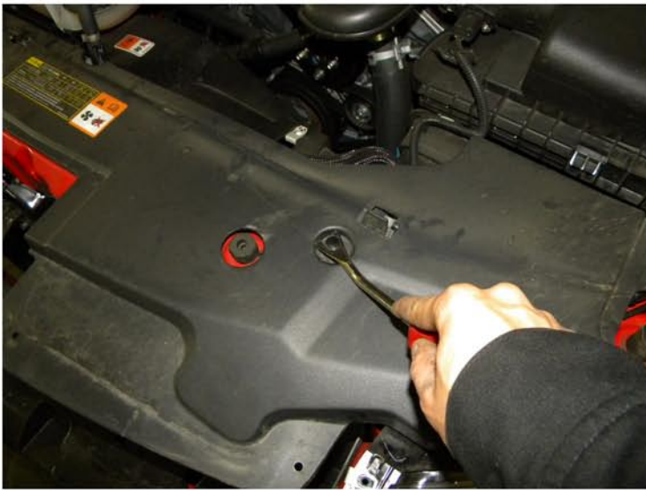
11. Remove the (4) plastic clips
