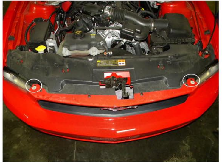
4. (2) 10mm bolts and (4) plastic clips locations
