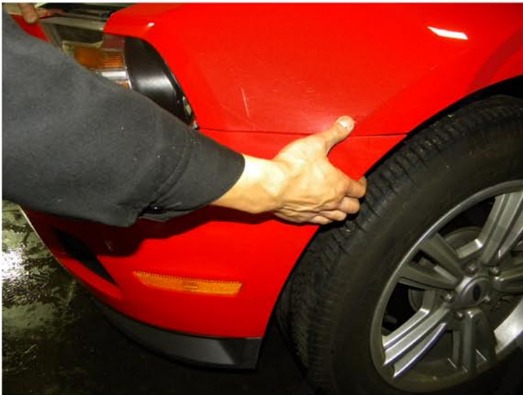
7. Pull on the side of the front bumper
