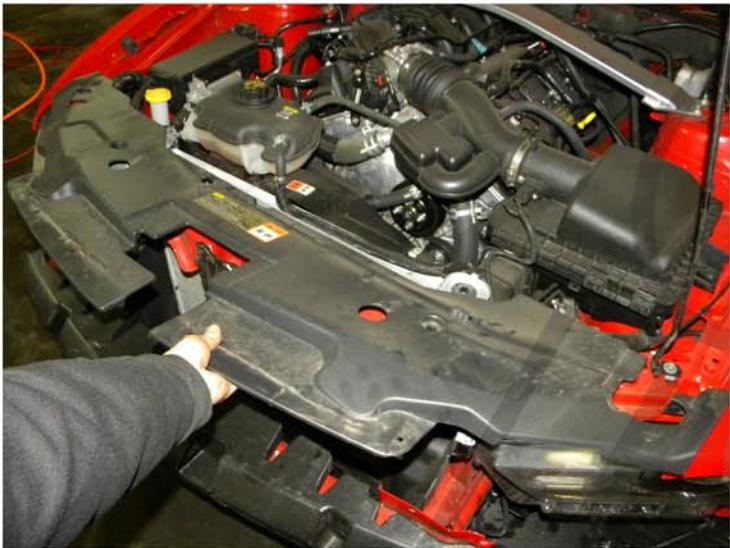
13. Remove the plastic radiator cover
