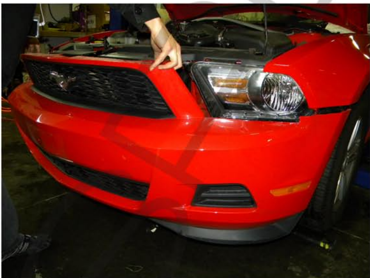
9. Remove the front bumper
