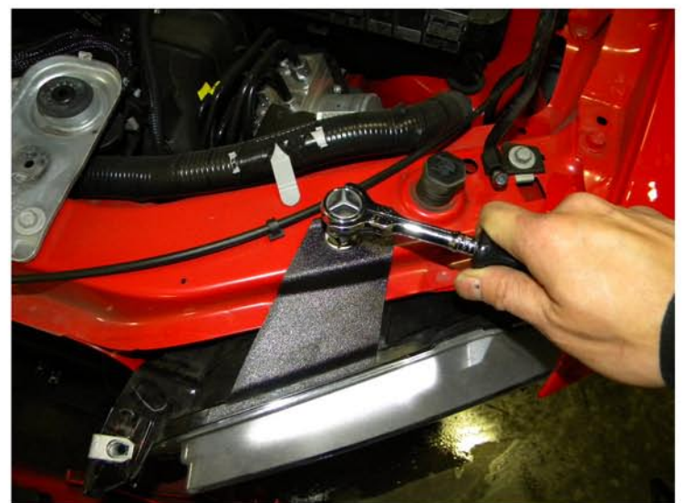
22. Tighten the 10mm bolt
