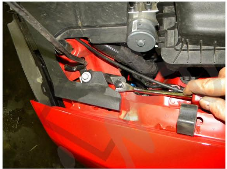
12. Remove the (4) plastic clips
