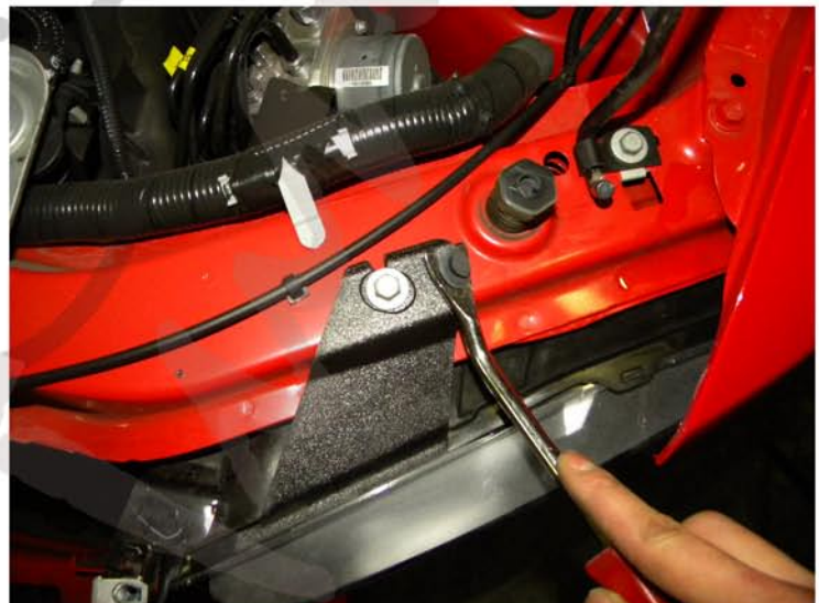
14. Remove the plastic clip
