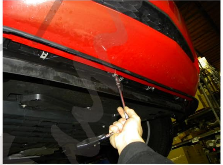
2. Remove the (4) 7mm screws
