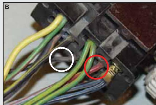
Locate single black wire or the red with yellow stripe wire in the headlight switch connector.
