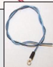
The loop connector on the end of the blue wire will attach to the accessory post on the back of the ignition switch. Secure the loop connector with the nut from the accessory post.
