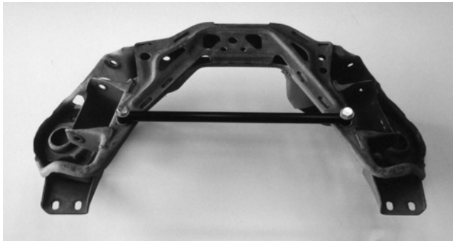
2-Point K-Member Brace placement on the K-member as viewed from the rear of the car
