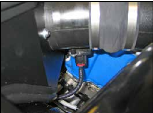
25. Reconnect the mass air sensor electrical connection.
