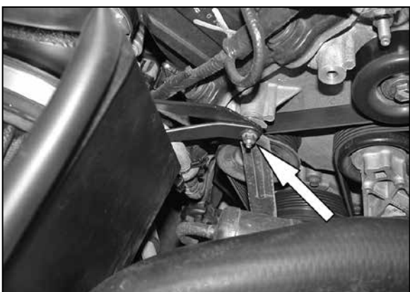
22. Slide the brackets onto the stud from step 11 and secure with the factory nut.
