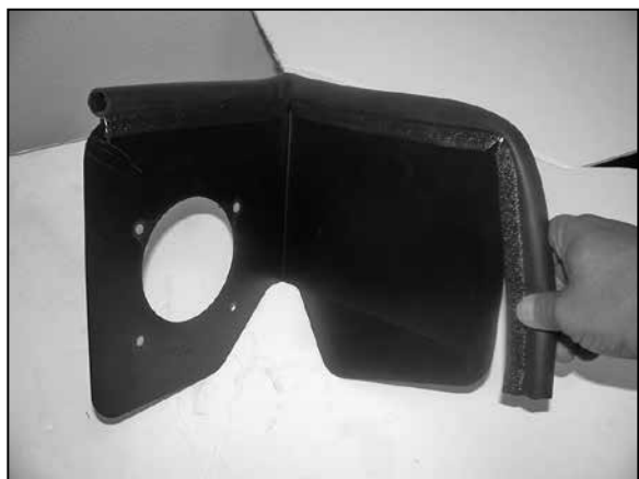
12. Install the trim seal onto the heat shield. NOTE: Some cutting and trimming will be necessary to achieve best fit.
