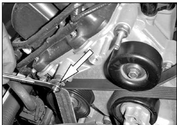
11. Loosen and remove the nut from the protruding stud on the engine. NOTE: Not all vehicles are equipped with a nut.
