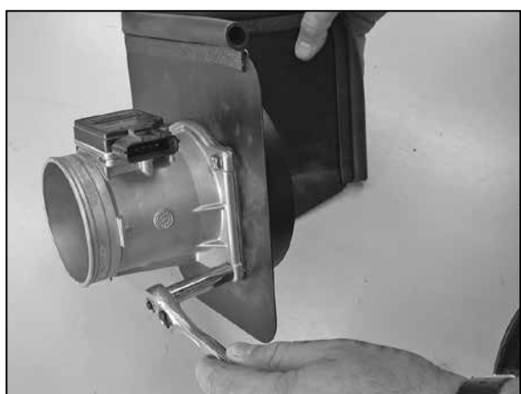
13. Assemble the mass air sensor, heat shield and adapter, using the gaskets and hardware provided as shown, but do not tighten completely at this time. NOTE: Do not install the hex bolts on the opposite side of flange. See next step.
