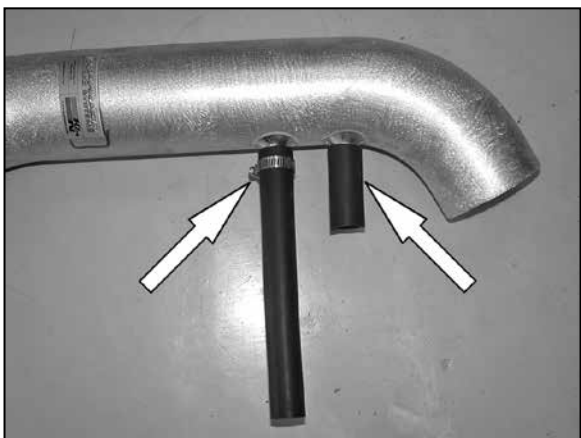
17. Install the provided hoses from the previous step onto the K&N® intake tube and secure with the provided hose clamps as shown. NOTE: Before installing the silicone hoses, inspect the inside of the tube for any debris, then clean the inside out with water and a towel. Inspect the tube one more time before proceeding to the next step.
