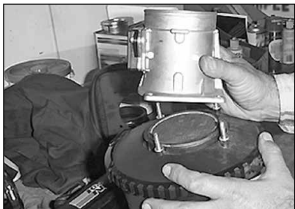
10. Remove the mass air sensor from the air cleaner. NOTE: The screen will not be reused.
