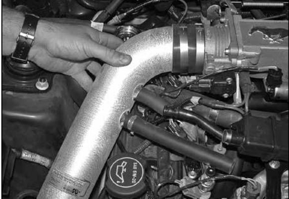
21. Install the complete K&N® intake assembly into the vehicle and slide the tube into the silicone hose on the throttle body as shown.
