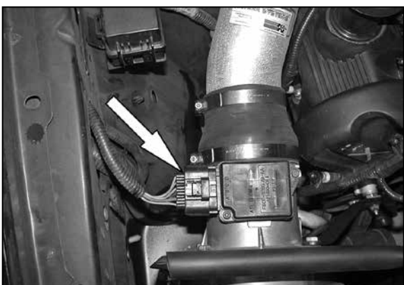
24. Reconnect mass air sensor electrical connection as shown.
