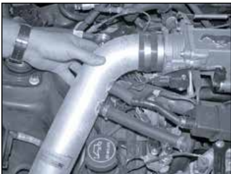
24. Install the complete K&N intake assembly into the vehicle and slide the tube into the silicone hose on the throttle body as shown.
