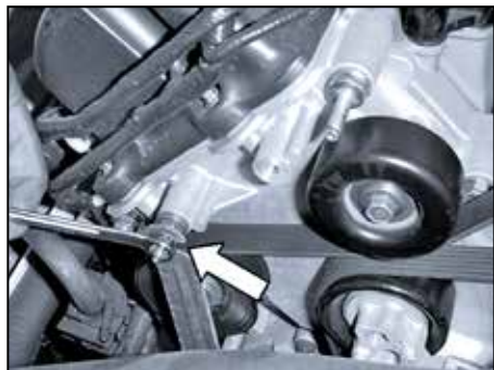
13. Loosen and remove the nut from the protruding stud on the engine. NOTE: Not all vehicles are equipped with a nut.
