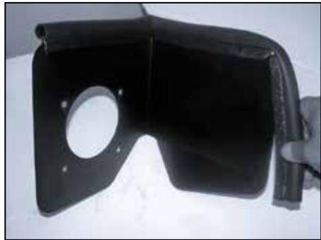
14. Install the trim seal onto the heat shield. NOTE: Some cutting and trimming will be necessary to achieve best fit.
