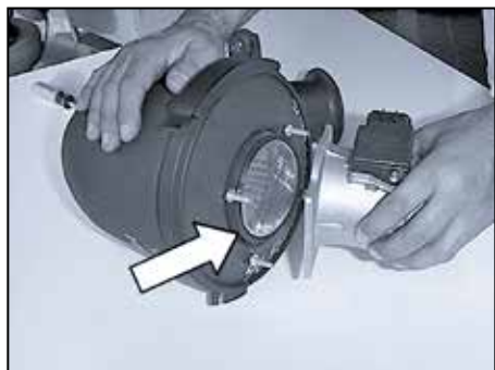
12. Remove the mass air sensor from the air cleaner. NOTE: The screen will not be reused.
