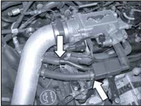
26. Reconnect the vent hoses to the K&N intake tube as shown and tighten hose clamps.
