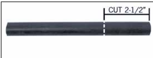
18. Mark and cut 2-1/2" from the provided silicone hose as shown
