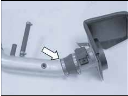
22. Install the K&N intake tube onto the mass air sensor and snug the hose clamps, but do not tighten completely at this time.
