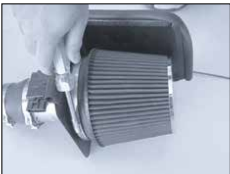
23. Install the K&N air filter onto the filter adapter and secure with the provided hose clamp as shown.
