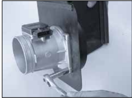
15. Assemble the mass air sensor, heat shield and adapter, using the gaskets and hardware provided as shown, but do not tighten completely at this time. NOTE: Do not install the hex bolts on the opposite side of flange. See next step.
