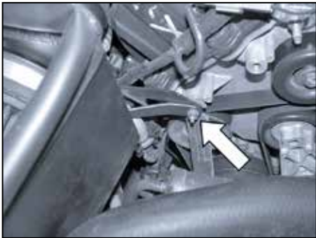
25. Slide the brackets onto the stud from step 13 and secure with the factory nut.
