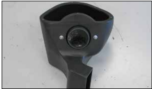
11. Install the filter adapter into the K&N® airbox and secure with the provided hardware.
