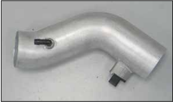
18. Install the 90° vent fitting into the K&N® intake tube as shown. NOTE: Plastic NPT fittings are easy to cross thread. Install the vent fitting “hand” tight, then turn it two complete turns with a wrench.
