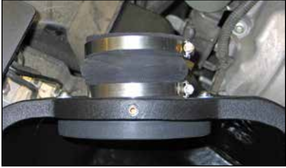
19. Install the silicone hump hose (08699) onto the filter adapter and secure with the provided hose clamp.
