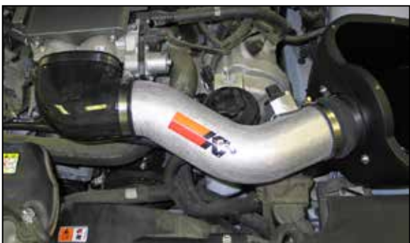
22. Install the K&N® intake tube assembly into the silicone hose on the filter adapter, and then into the 90° hose attached to the throttle body. Adjust the tube and hose for proper fit, then tighten the hose clamps.
