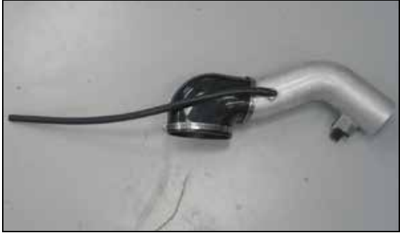
21. Install the provided crankcase vent hose onto the 90° fitting installed into the K&N® intake tube.
