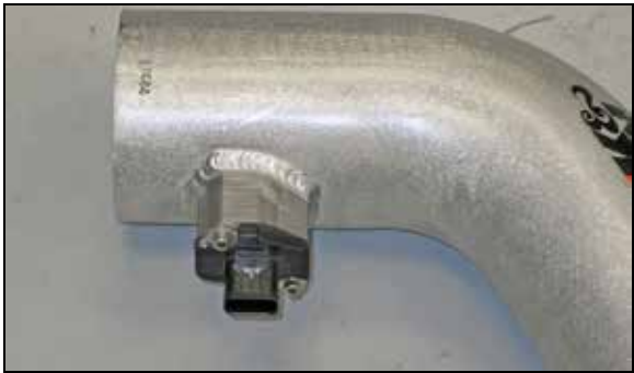
17. Install the mass air sensor into the K&N® intake tube and secure with the provided hardware.
