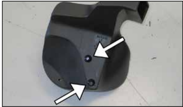
12. Install the two provided mounting studs onto the bottom of the K&N® airbox using the provided hardware.
