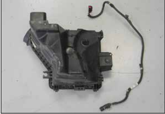
26. Remove the mass air sensor wiring harness from the factory airbox.
