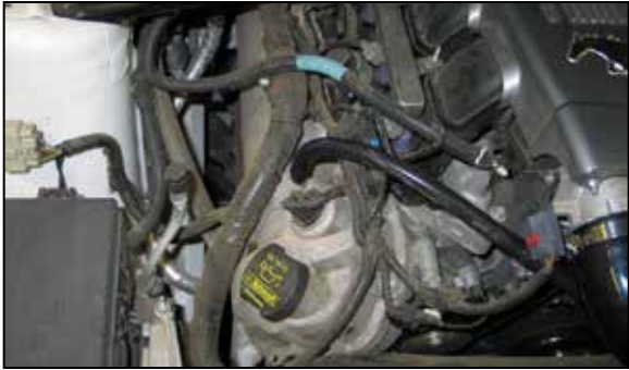
23. Connect the crankcase vent hose to the vent port on the valve cover.
