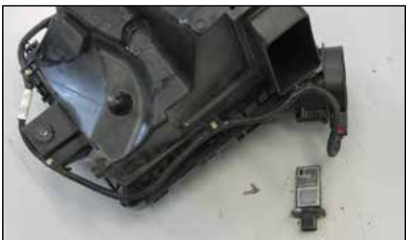
16. Remove the two screws securing the mass air sensor and then remove the mass air sensor from the factory airbox.
