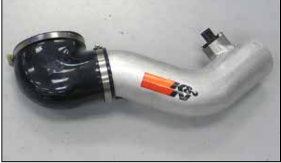
20. Install the 90° silicone hose onto the K&N® intake tube as shown. Do not tighten the hose clamp at this time.
