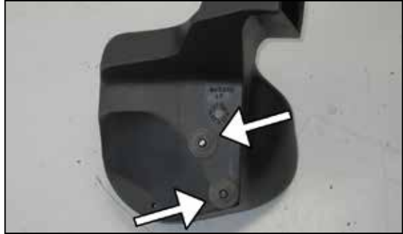
14. Install the two airbox mounting grommets to the mounting studs installed onto the K&N® airbox as shown.
