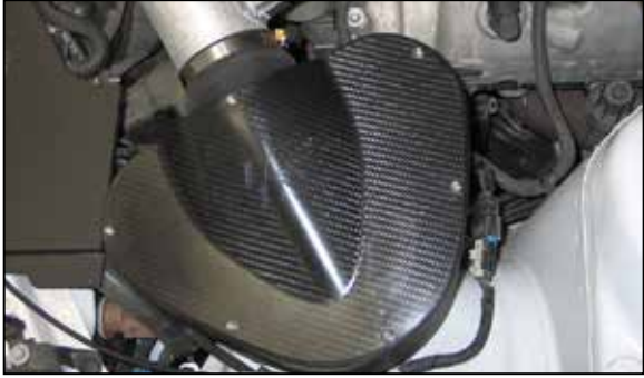
27. Connect the mass air harness to the vehicle harness, routing the mass air harness around the K&N® airbox. Connect the mass air harness to the mass air sensor.
