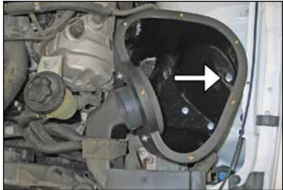
15. Set the K&N® airbox into position on the inner fender and secure to the factory mounting location with the hardware provided.
