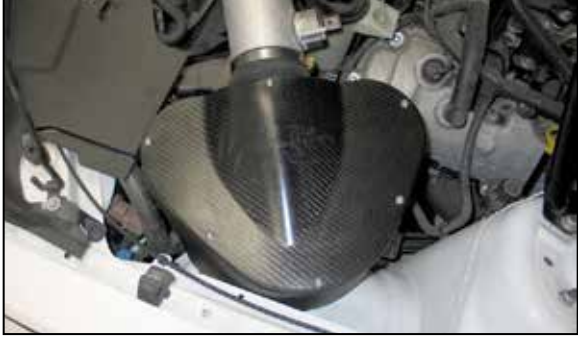
25. Install the airbox lid onto the airbox and secure with the provided hardware.
