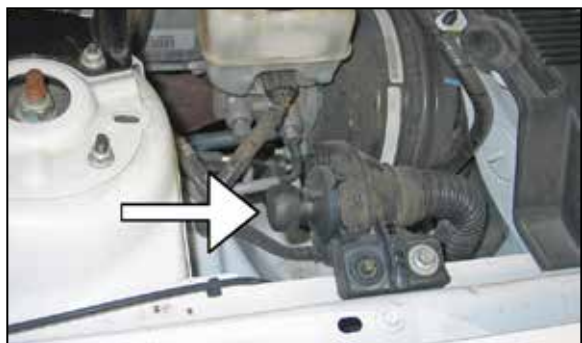
10. Install the provided cap plug onto the pulse drum as shown.
