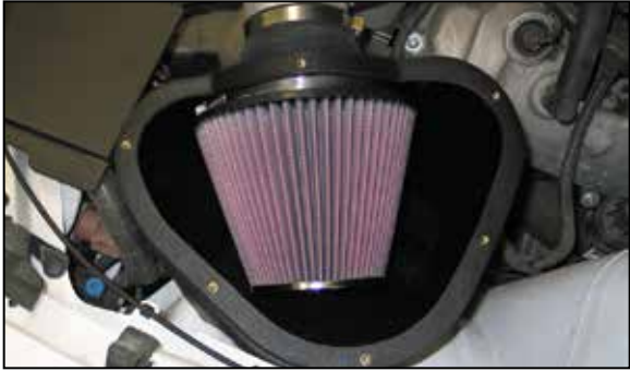
24. Install the K&N® air filter onto the filter adapter and secure with the provided hose clamp. NOTE: Drycharger® air filter wrap; part # RF-1048DK is available to purchase separately. To learn more about Drycharger® filter wraps or look up color availability please visit http://www.knfilters.com ®.
