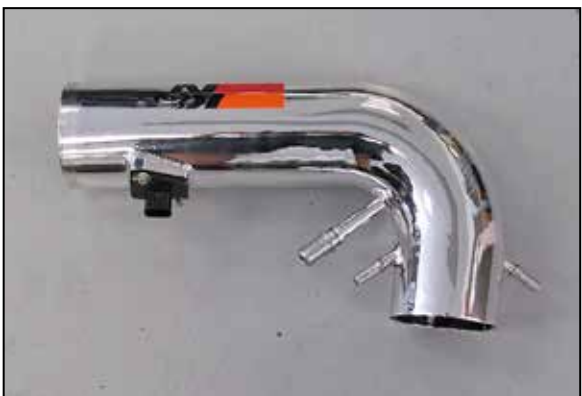
19. Install the mass air sensor into the K&N® intake tube and secure with the provided hardware.
