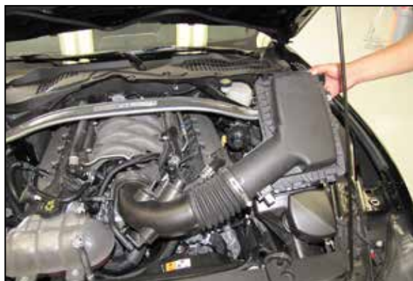
9. Loosen the hose clamp securing the intake tube to the throttle body and then remove the air filter assembly and intake tube from the engine compartment. NOTE: K&N Engineering, Inc., recommends that customers do not discard factory air intake.
