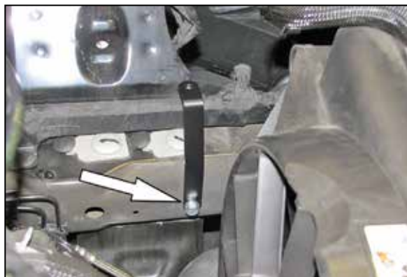
10. Install the heat shield mounting bracket (064325) onto the inner fender as shown using the provided hardware.
