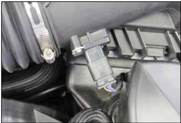
7. Release the locking tab and then disconnect the mass air sensor electrical connection.
