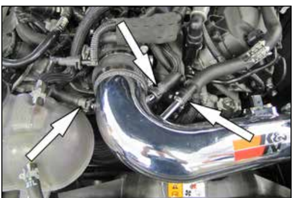
21. Connect the crank case vent, EVAP vent and idle by pass lines to the quick disconnect fittings installed into the K&N® intake tube. NOTE: On vehicles not equipped with an EVAP vent line, install the provided caplug #08215 onto the quick disconnect fitting.
