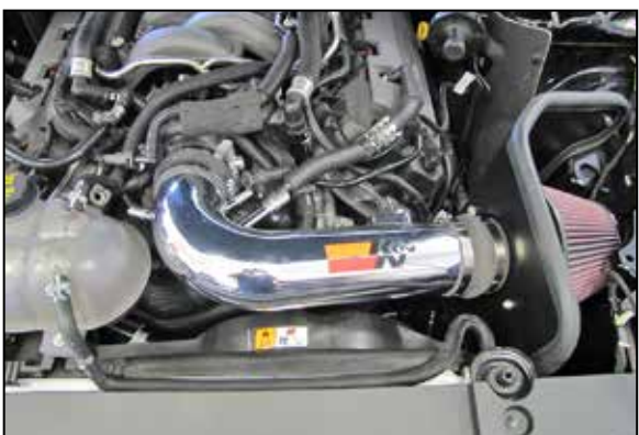
20. Install the K&N® intake tube into the hose at the filter adapter and then into the hose at the throttle body, adjust the tube and hoses for best fit and then secure with the provided hose clamps.
