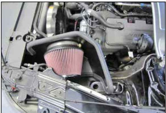
15. Install the K&N® air filter onto the adapter and secure with the provided hose clamp, then secure the heat shield and brackets to the air filter housing mounting location using the provided hardware. NOTE: Drycharger® air filter wrap; part # 22-8049DK is available to purchase separately. To learn more about Drycharger® filter wraps or look up color availability please visit http://www.knfilters.com ®.
