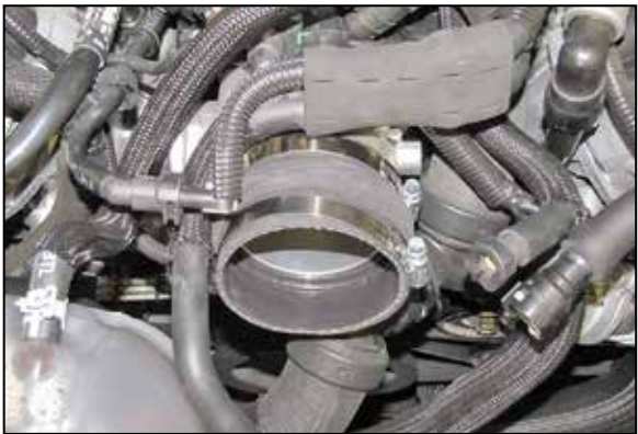
17. Install the provided hump coupler (08699) onto the throttle body and secure with the provided hose clamp.
