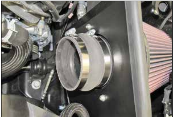
16. Install the provided hump coupler (08699) onto the filter adapter and secure with the provided hose clamp.
