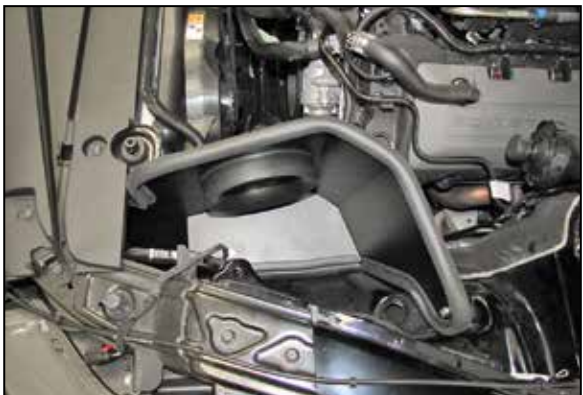
14. Set the heat shield onto the mounting bracket installed in step #9 and secure with the provided hardware. NOTE: Do not secure the top bracket at this time.
