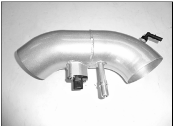
15. Install the provided 90° fitting into the K&N® intake tube. Remove the mass air sensor from the factory housing and install it into the K&N® intake tube using the provided hardware. NOTE: Plastic NPT fittings are easy to cross thread. Install the vent fitting "hand" tight, then turn it two complete turns with a wrench.
