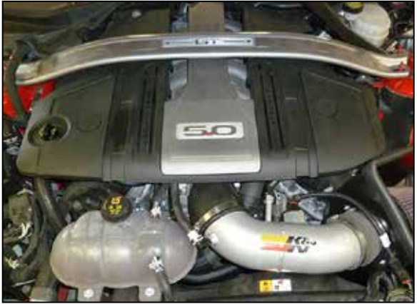
20. Reinstall the engine cover and secure with the factory hardware, reinstall the nut covers. Reinstall the strut tower brace and secure with the factory nuts.
