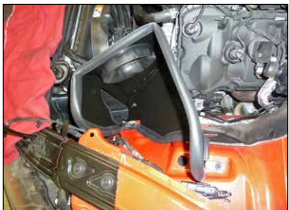
12. Install the heat shield assembly onto the inner fender and secure with the provided hardware. NOTE: The K&N fresh air duct should be around the factory inlet duct.
