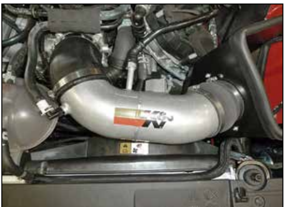
16. Install the intake tube into the coupler at the throttle body and onto the coupler at the filter adapter, adjust the tube for best fit and then secure the tube to the coupling hoses with the provided hose clamp. Connect the EVAP and crank case vent lines to the fittings installed into the K&N® intake tube.
