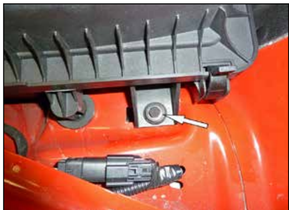
7. Remove the bolt that secures the air filter housing to the inner fender and then remove the lower air filter housing from the vehicle. NOTE: K&N Engineering, Inc., recommends that customers do not discard factory air intake.
