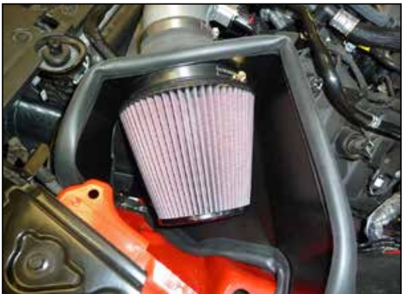
19. Install the K&N® air filter onto the filter adapter and secure with the provided hose clamp. NOTE: Drycharger® air filter wrap; part # RF-1042DK is available to purchase separately. To learn more about Drycharger® filter wraps or look up color availability please visit http://www.knfilters.com® .
