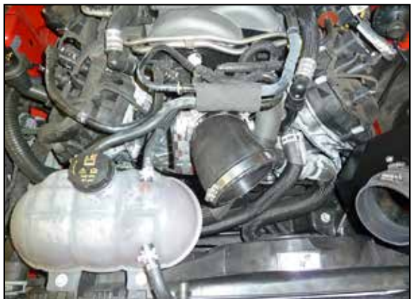
14. Install the provided angled coupler hose (5-1100) onto the throttle body and secure with the provided hose clamp.
