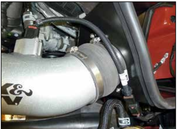
17. Reconnect the mass air sensor electrical connection using the provided extension harness.
