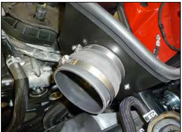
13. Install the provided hump coupler (08418) onto the filter adapter and secure with the provided hose clamp.
