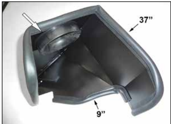
9. Install the provided edge trim onto the K&N® heat shield as shown. Install the air filter adapter into the heat shield and secure with the provided hardware.
