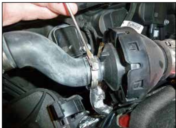
6. Release the one-time use clamp that secures the sound tube to the drum and then disconnect and remove the sound tube from the vehicle.
