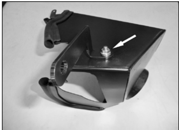
10. Install the provided mounting bracket (064357) onto the heat shield and secure with the provided hardware.
