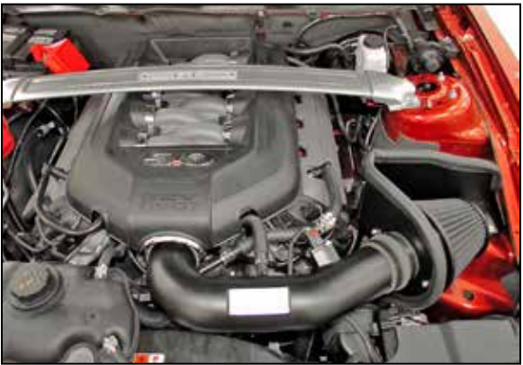
28. Reconnect the vehicle's negative battery cable. Double check to make sure everything is tight and properly positioned before starting the vehicle.
