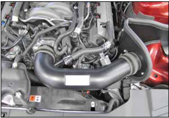
22. Install the K&N® intake tube into the silicone hoses, align for best fit and then secure with the provided hose clamps.
