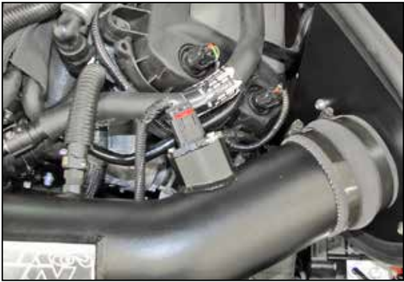
24. Connect the mass air sensor electrical connection.
