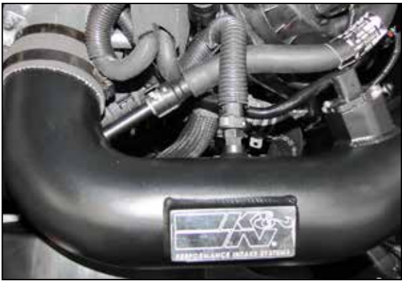
23. Connect the crank case vent line and EVAP vent line if equipped as shown.
