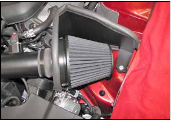
27. Install the K&N® air filter and secure with the provided hose clamp.
