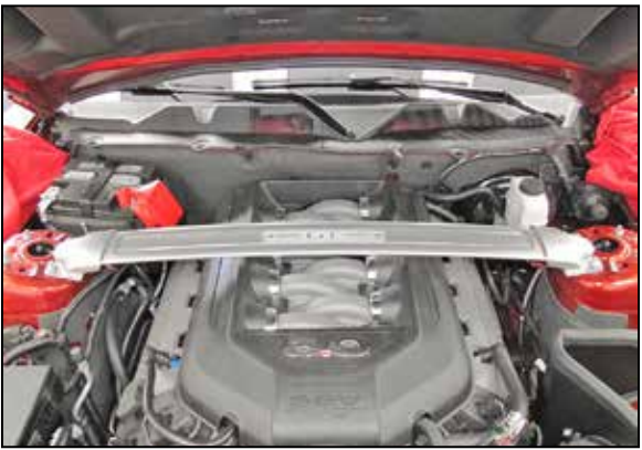
26. Reinstall the strut tower brace and secure with the factory nuts.
