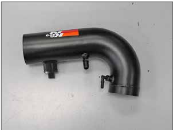
20. Install the two vent fittings into the K&N® intake tube as shown.
