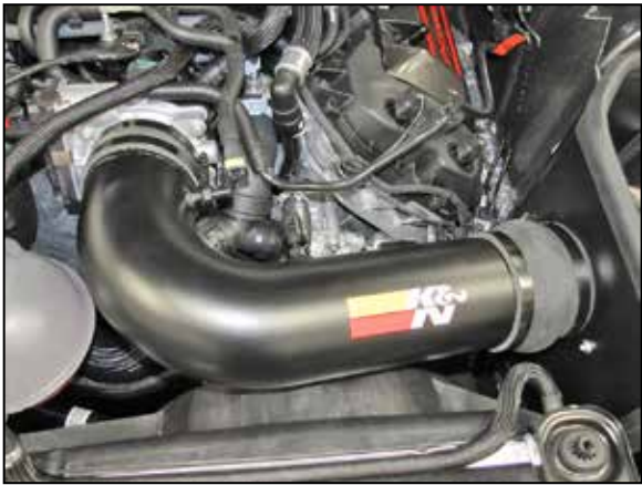
21. Install the K&N® intake tube into the coupler at the filter adapter and then into the coupler at the throttle body, adjust the tube for best fit and then secure with the provided hose clamps.
