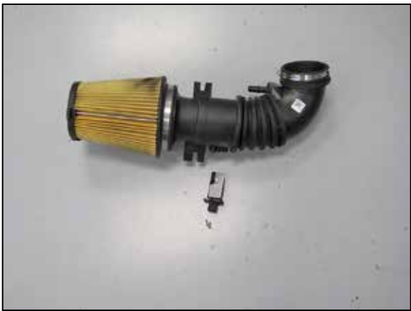
18. Remove the mass air sensor from the factory intake tube.
