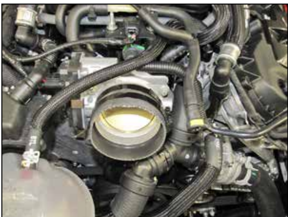
17. Install the provided coupler (08618) onto the throttle body and secure with the provided hose clamp.
