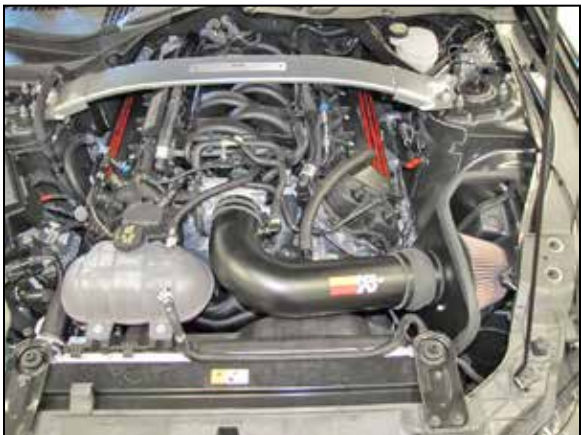
26. Reconnect the vehicle's negative battery cable. Double check to make sure everything is tight and properly positioned before starting the vehicle.
