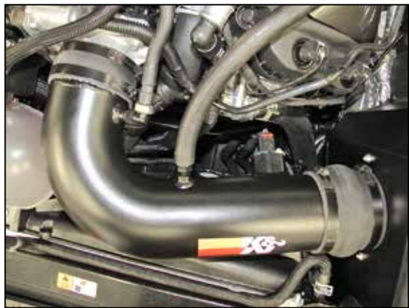
25. Reconnect the mass air sensor electrical connection.
