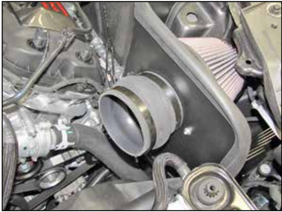
16. Install the provided hump coupler (08418) onto the filter adapter and secure with the provided hose clamp.
