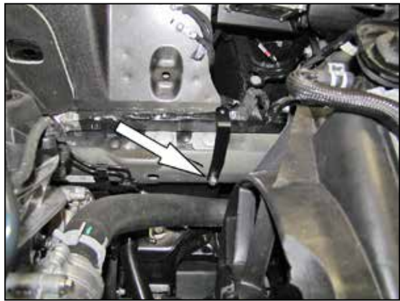
10. Install the heat shield mounting bracket (064325)
