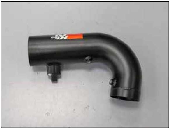
19. Install the mass air sensor into the K&N® intake tube and secure with the provided hardware.
