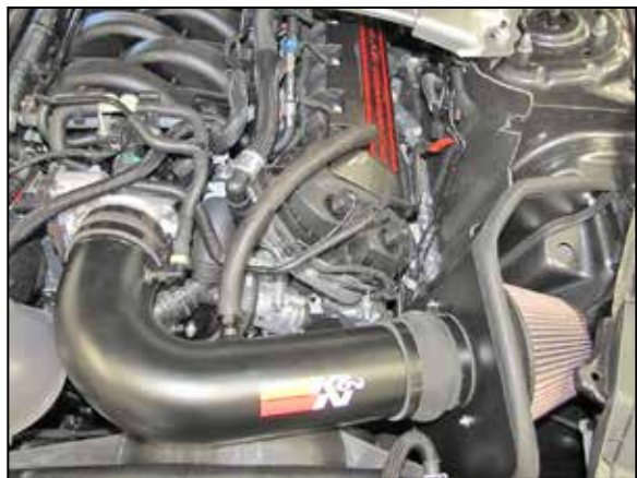
24. Install the crank case breather hose onto the valve cover port using the quick disconnect fitting and then install the open end onto the fitting installed into the K&N® intake tube.
