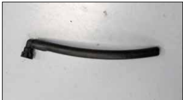
23. Install the provided 5/8 quick disconnect fitting into the provided crank case breather hose.
