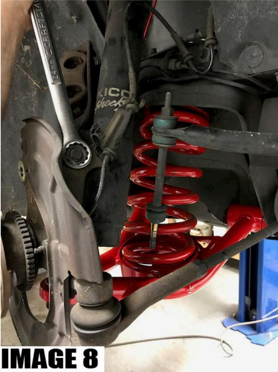
19. Using the E8 socket, install ABS sensor and clip ABS wires back in.
