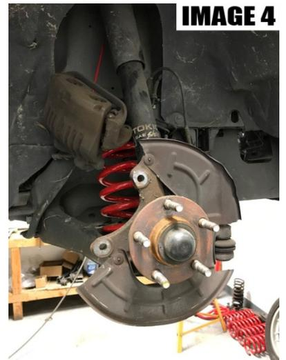
5. Using the E8 socket, remove the ABS sensor.
