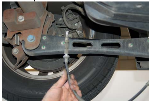
Pull cable through control arm
