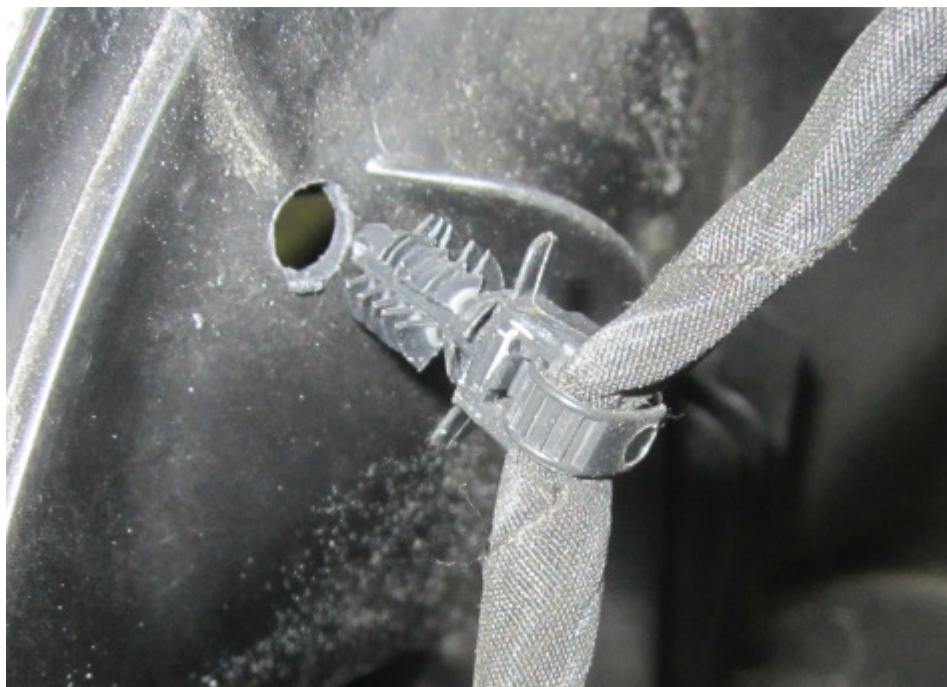
Drill hole for harness retainer.
