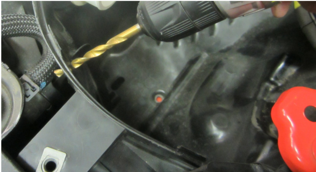
Drill hole for harness retainer.
