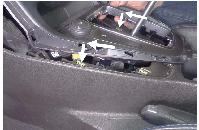
60. Install the power panel with a “forward-then-down” motion (the reverse of Steps 21 and 20). First move the panel forward, inserting its alignment tabs in their slots in the center dash. Then push it downward, snapping it into the 4 clips in the center console.
