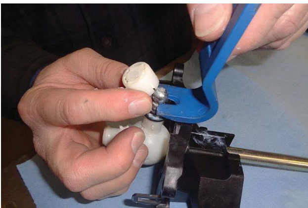
33. Pull the side pivot cup off of the side pivot ball.
