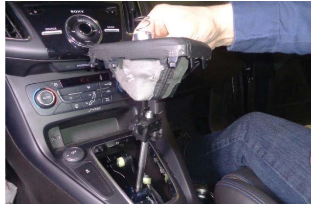
65. Slip the assembled boot and reverse lockout sleeve onto the shift lever.
