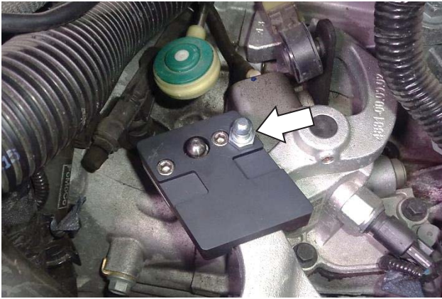
43. Apply medium strength thread-locking fluid to the one of the ball studs (6) and install it in the shift plate.
