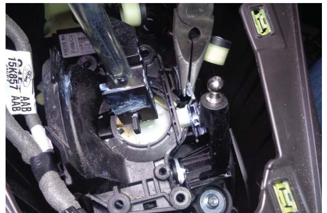
30. Use pliers to lift the top leg of the centering spring up off the rubber grommet on the side shaft.
