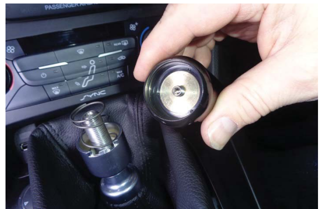
67. Install the set screw (3) in the shift knob (4), leaving 2-3 threads exposed.
