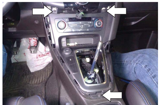
61. Install and tighten the 3 power panel screws.
