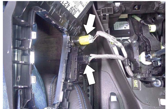
23. Disconnect the yellow (12V) and black (traction control) connectors.
