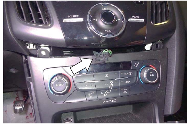
59. Ensure that the center panel bezel plug is exposed and accessible before reinstalling the power panel.
