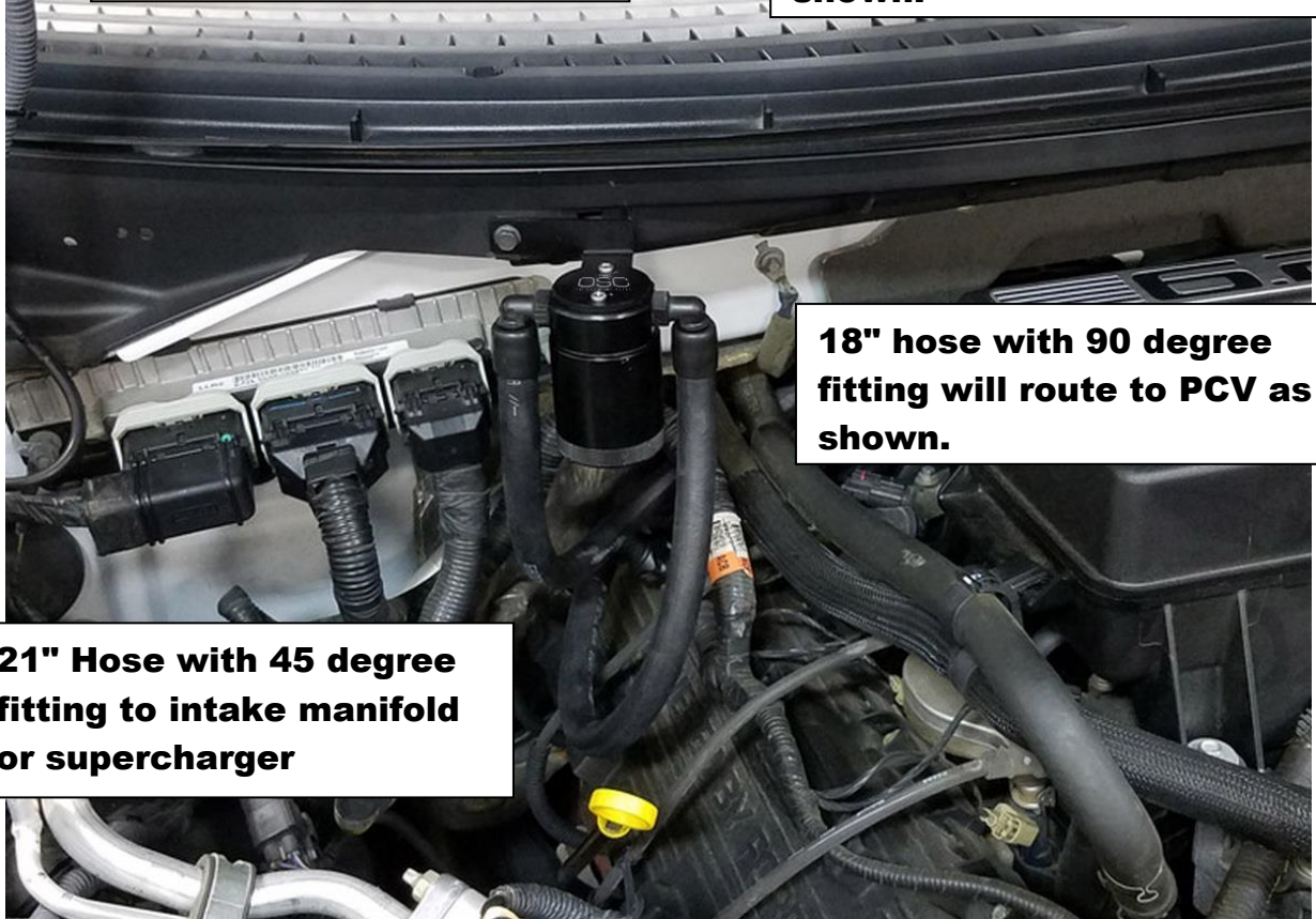
18" hose with 90 degree fitting will route to PCV as shown.
