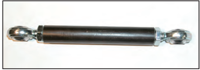
Correct: The rod ends are aligned.
