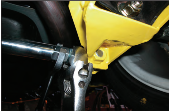
Incorrect: The rod ends are not aligned.
