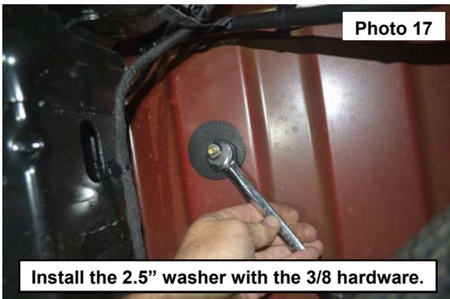
**Install the 2.5" washer with the 3/8 hardware.**
