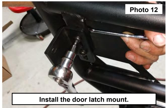
12. Install the door latch onto the latch plate with the latch release pointed up using 2 of the supplied 6mm x 25mm button head bolt, (2) 6mm flat washers. Snug hardware using a 4mm allen wrench. **See Photo 13.** If needed install the shim plates between the latch plate and the tube door to allow the latch to function properly.
