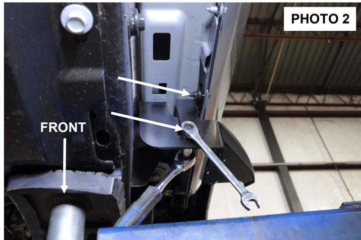
4. Install the rear step bracket pointing toward the front with the supplied 8mm lock nuts, 8mm x 30mm bolts, lock washers and flat washers. **See Photo 3.** Do not fully tighten using a 13mm socket.
