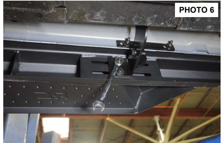
8. Adjust the step to the body and tighten the body mount brackets in using a 13mm socket / wrench.
