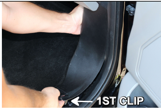
Remove kick panel. First pull upward, then backward, 5
