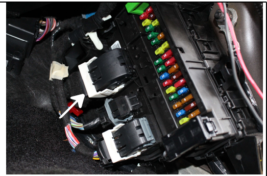
Press tab while sliding bar to the side to unplug connector. 6
