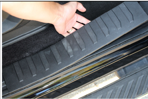
Remove passenger side door sill plate carefully. 4
