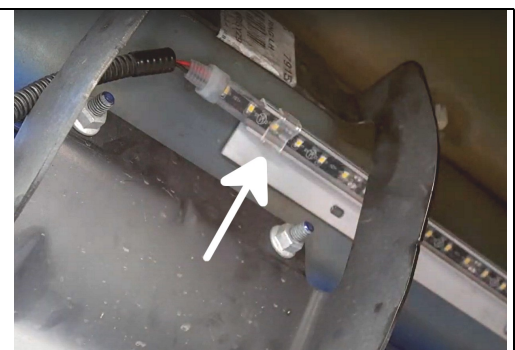
Install retaining clips on either end of rail. 3
