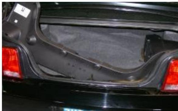
3. Remove 11mm nuts securing taillight housing to the vehicle, 3 per taillight housing. Unplug wiring harness (one connection per side). Push grommet (one per side) with wiring harness through the sheet metal from inside to outside of trunk. Remove taillight housings from vehicle.
