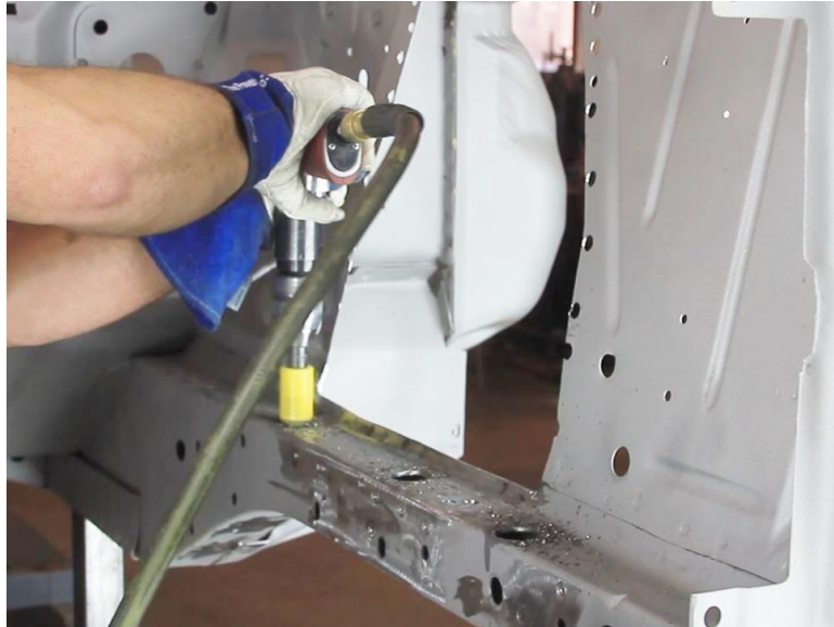
Figure 9 – Drill-Out Top Framerais
