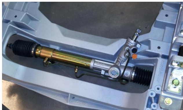
Figure 40 - Installed Rack & Pinion
