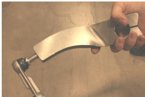
Figure 43 – Pre-assemble ARB Endlinks
