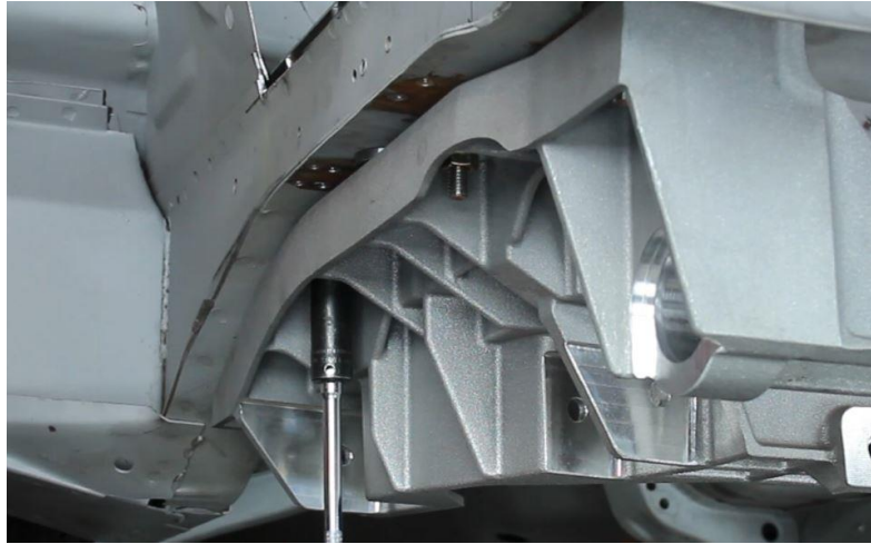
Figure 15 - Install Aluma-Frame Cradle Hardware
