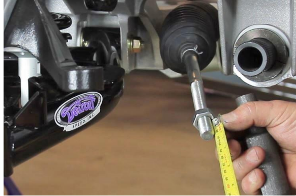
Figure 41 – Install Outer Tie Rods
