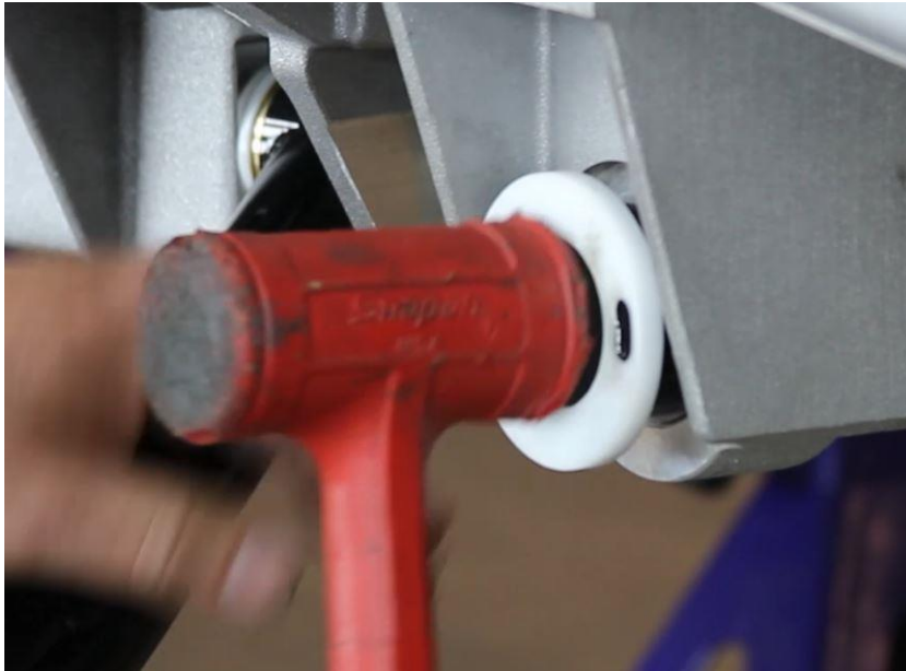
Figure 22 - Install ARB Bushings
