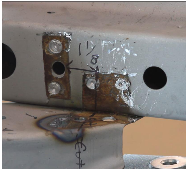
Figure 4 - Trim Framerail Brace
