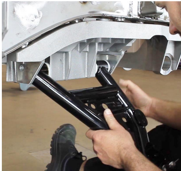
Figure 20 – Install Lower Control Arms
