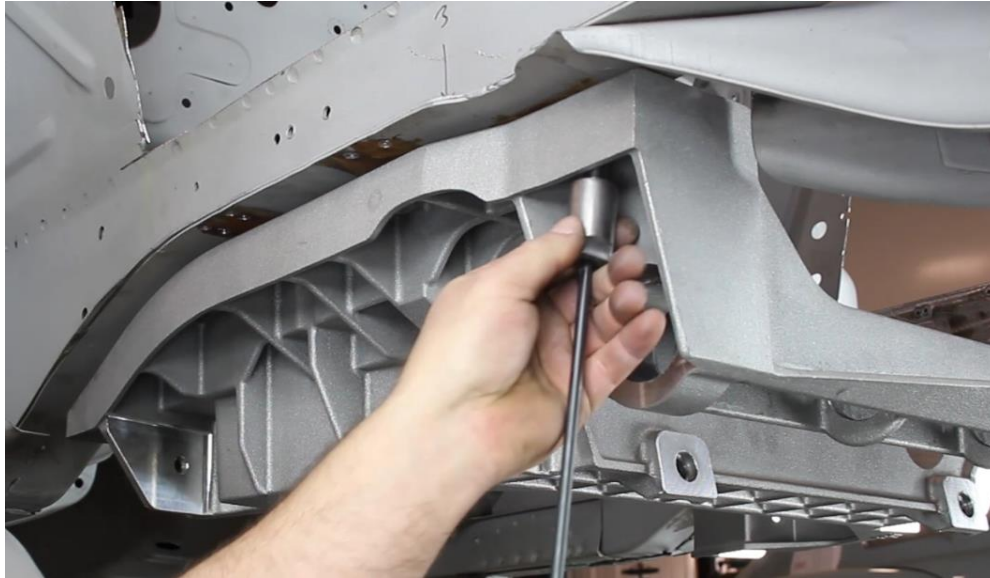
Figure 7 - Locate Aluma-Frame Mounting Holes
