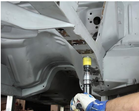
Figure 8 - Drill-Out Bottom Frameraills
