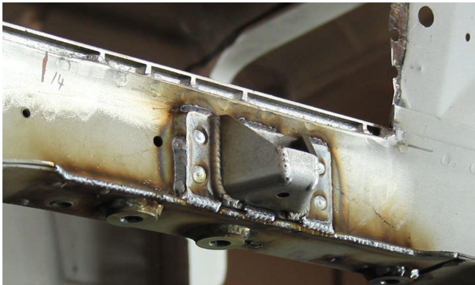
Figure 19 - Weld Jounce Bumper Bracket
