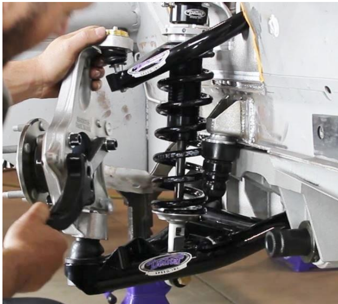
Figure 37 - Install Spindle Assembly
