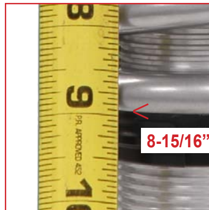
Measure the bottom end of the spring.
